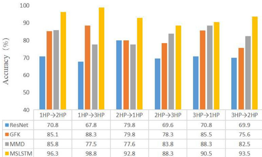
Fig. 8. The diagnosis accuracy of transfer learning under the condition of variable load scenario
