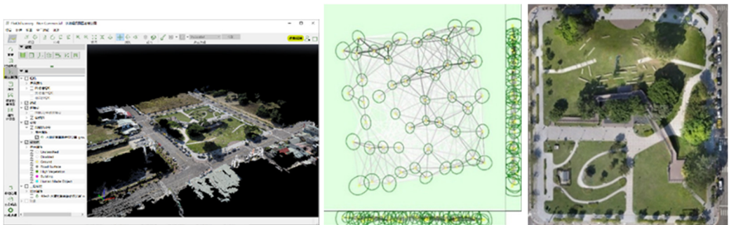
Fig. 3. Point cloud model creation and image matching from a quadcopter unmanned aerial vehicle (UAV)
