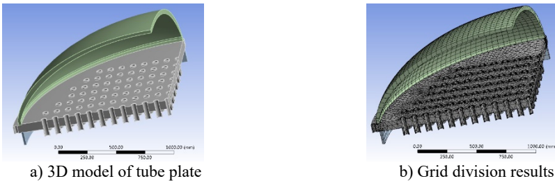
Fig. 7. Finite element model of tube plate
