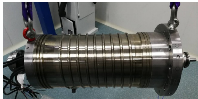
Fig. 3. Schematic diagram of the free mode of the electric spindle
