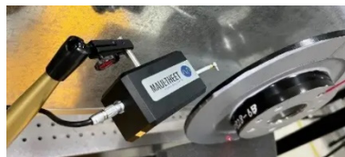
Fig. 6. Modal testing scheme
