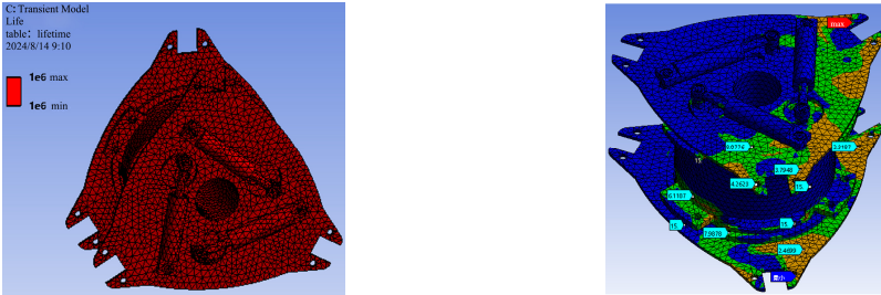
Fig. 10. Powertrain safety factor and fatigue life diagram
