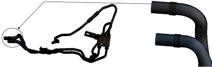
Fig. 2. The result of finite element mesh division
