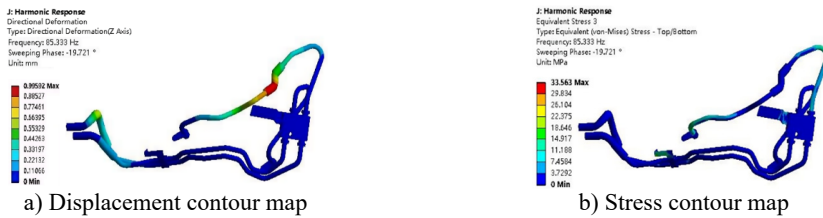
Fig. 6. The harmonic response analysis results under 4 g acceleration
