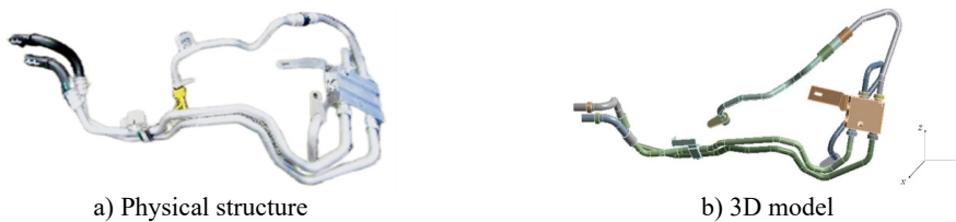
Fig. 1. Structure and modeling of hydraulic pipeline
