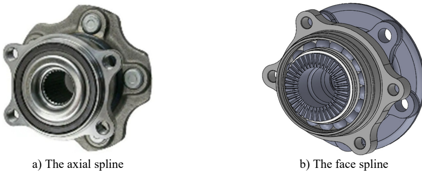
Fig. 1. Hub bearing with two types of spline
