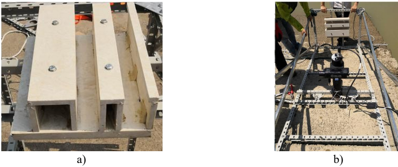
Fig. 6. a) Frontal view of the homemade upright bank wall model, b) sonar and model fixed to the measurement stand
