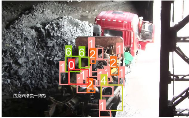
b) More detailed rendering of scrap classification Fig. 4. Practical effect of steel scrap classification
