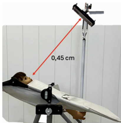
Fig. 2. Macri. Baby positioned at a tilt of 220 and wrapped with a Velcro band at a distance of 45 cm. Full-size photo with direct measurement from the diagonal between the baby's lips to the center point of the cell phone holder
