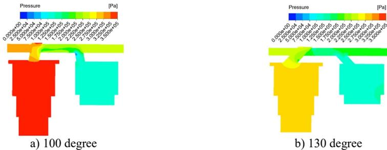
Fig. 9. Response results of pressure field under different bending angle
