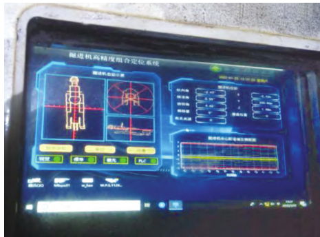
Fig. 20. Position and attitude monitoring of roadheader fuselage
