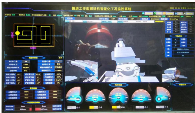
Fig. 22. Monitoring of motion trajectory of cutting head
