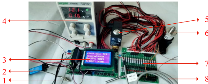
Fig. 13. PID self-tuning experimental platform for pulsating vacuum sterilizers: 1 – resistance wire; 2 – ST-LINK STM32 emulator programmer; 3 – sterilizer temperature control panel; 4 – control system power supply; 5 – electromagnetic valve; 6 – pressure sensor; 7 – signal expansion board; 8 – PT100 temperature sensor
