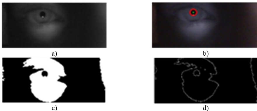
Fig. 6. a) Pupil image acquired by the camera and b) detection of circles made by the software; c), d) images in black/white and contour detection
