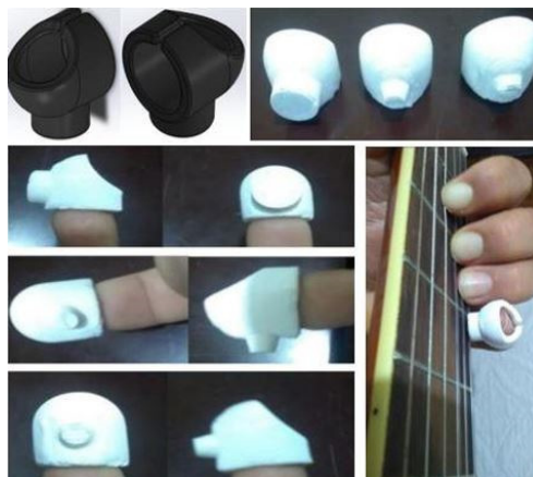
Fig. 5. The image displays the 3D modeling of the thimble from the front and back, as well as the finished pieces. Three types of thimbles for distal phalanges are presented, along with the practical application of the thimble on a string instrument, mainly a guitar
