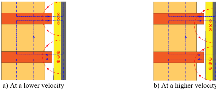
Fig. 8. Schematic diagram of induced magnetic field of eddy currents at different speeds (Reproduced with permission from [Analytical modeling of permanent magnet linear eddy current brake using magnetic equivalent circuit method], IOS Press, 2022)
