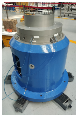
Fig. 12. Assembled aerostatic rotary table
