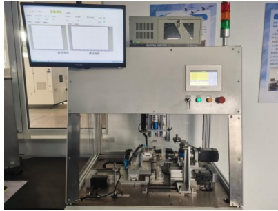
Fig. 5. Physical picture of bearing flexibility detection system
