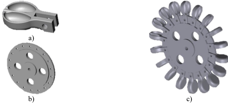
Fig. 4. a) Bucket design, b) runner design, c) Pelton turbine design
