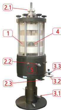
Fig. 4. GDS dynamic triaxial shear tester: 1 – pressure chamber; 2.1 – load sensor; 2.2 – pore pressure sensor; 2.3 – displacement sensor; 3.1 – axial pressure controller; 3.2 – confining pressure controller; 3.3 – back pressure controller; 4 – top cap of the sample; 5 – base of the sample
