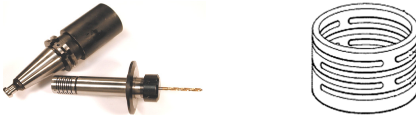
a) Photograph of an SVDH with an integrated elastic element b) An elastic element with openings
