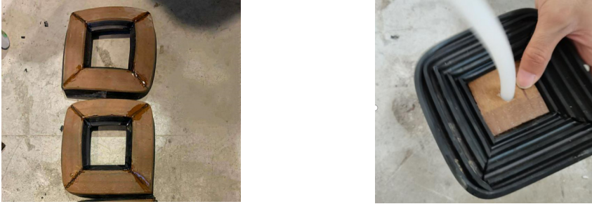
Fig. 2. Annular water-stop with hose fitting surface treatment
