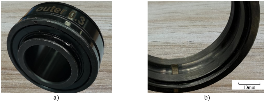
Fig. 10. Experimental bearing, a) defective bearing ER-16k, b) fabricated defect on outer raceway
