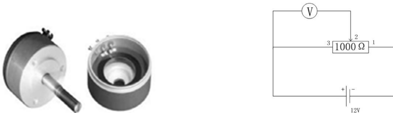
Fig. 5. Shape and working principle of the potentiometer
