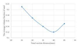
Fig. 5. Curve of sand volume fraction at different sand suction distances
