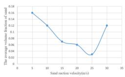
Fig. 7. Curve of sand volume fraction at different suction velocity
