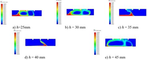
Fig. 4. Sand distribution at different sand suction distances
