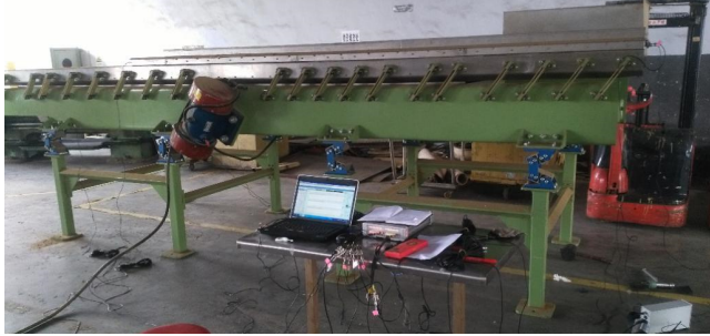
Fig. 8. Field diagram of double-layer vibrating screen machine test
