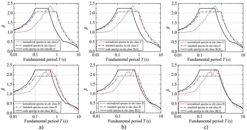
**Fig. 4.** Standard response spectra of NFPL long-period ground movements and code design spectra:
