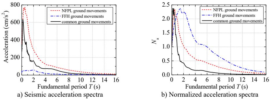
**Fig. 1.** Acceleration response spectra
