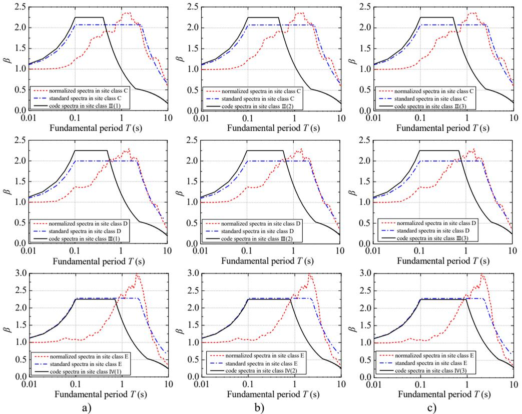
**Fig. 5.** Standard response spectra of FFH long-period ground movements and code design spectra: a) the first design earthquake group; b) the second design earthquake group; c) the third design earthquake group
