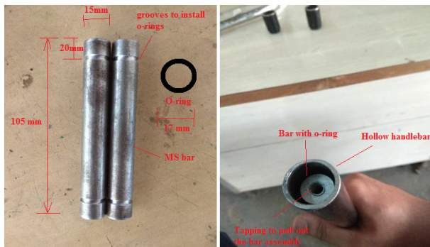
Fig. 1. Tuned mass damper
