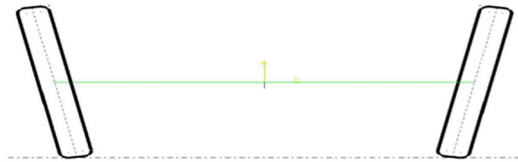
Fig. 2. Positive camber (front view)
