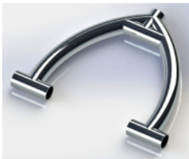
Fig. 12. A-equivalent front lower wishbone design
