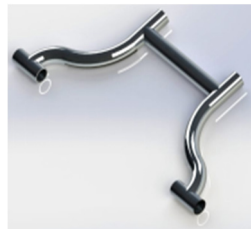
Fig. 13. H-equivalent rear lower wishbone design
