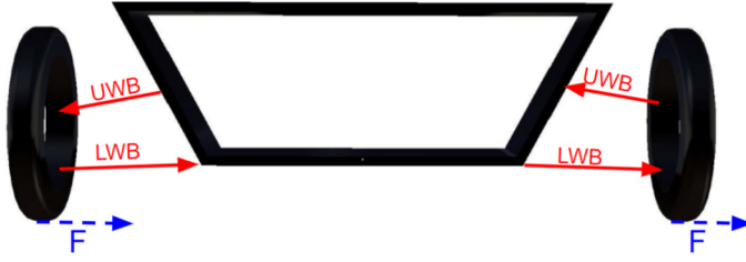
Fig. 8. Skeleton sketch of Wishbones (WB) mounting
