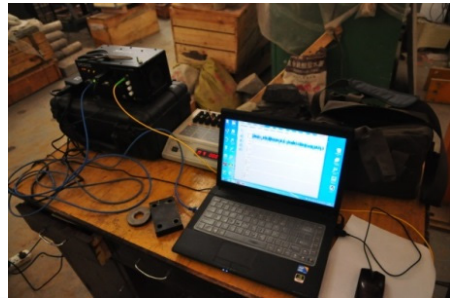
Fig. 11. Fiber Bragg grating dynamic signal acquisition instrument
