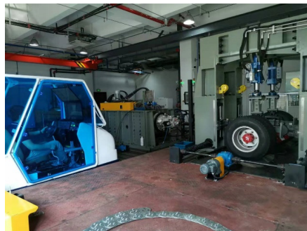
Fig. 1. Road load simulation system of vehicle drivetrain system based on dynamometer
