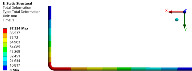
Fig. 3. Pipe thermal deformation
