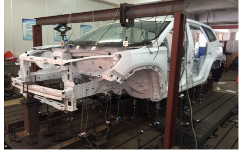
Fig. 10. Torsional stiffness test
