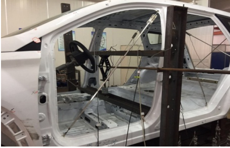
Fig. 9. Bending stiffness test
