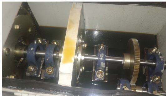
Fig. 1. Experimental setup- miniature wind turbine planetary gearbox
