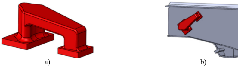
Fig. 5. A node for wagon fastening to the deck of the railway ferry a) general view; b) allocation on the draw bar
