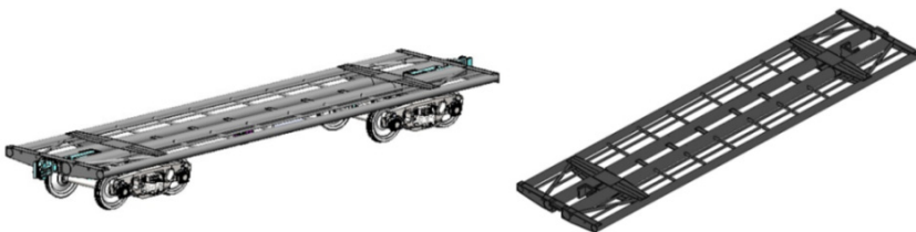
Fig. 2. Computer models of railway wagons whose bearing elements of bodies are made of round cross-section pipes: flat wagon
