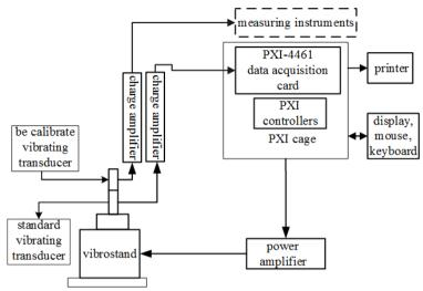
Fig. 1. Hardware architecture of vibration standard device
