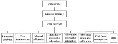
Fig. 2. Software architecture of vibration standard device
