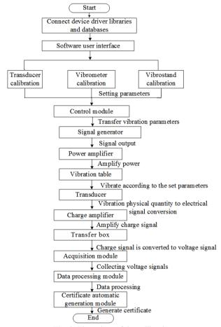
Fig. 3. Flow chart of the calibration
