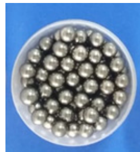
Fig. 3. Container with particle damper
