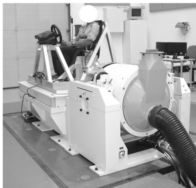
Fig. 2. Test bench during simulation of the horizontal vibration exposure
