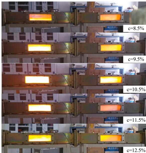
Fig. 10. Flame propagation process (electrode ignition) to show the bright orange flame
