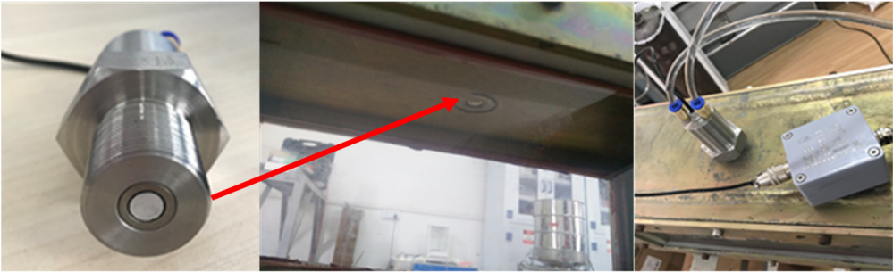
Fig. 7. The sensor used for the high-frequency water-cooled pressure transmitter
