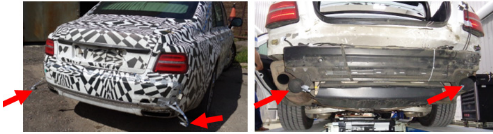
Fig. 2. Microphones at the left and right sections of exhaust pipes (a complete set with a rear bumper and end inserts of exhaust system)
