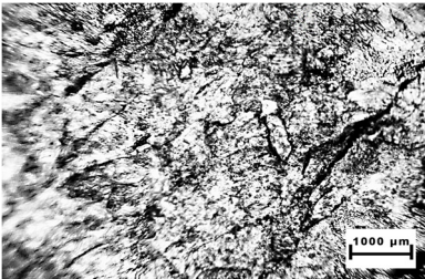
Fig. 6. Surface of metal chips after impact in a hammer mill at 20x magnification
