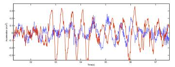
Fig. 2. The vertical accelerations of the passive seat suspension measured at floor (.....) and seat (\_\_\_\_)
