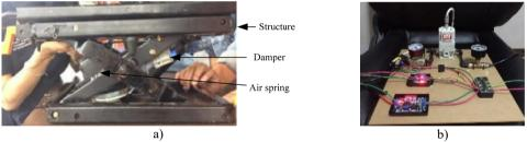
Fig. 5. a) Seat structure, b) air spring control valve
