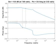
Fig. 13. Bode plot of the closed loop frequency response for maximum stiffness
