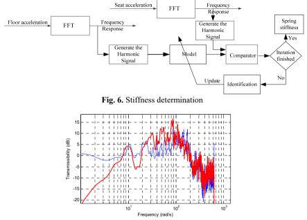
Fig. 7. Open loop transfer function (left) by varying the stiffness
