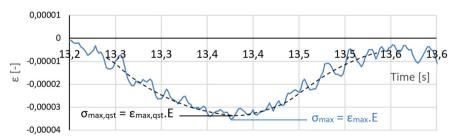
Fig. 3. Determining maximum dynamic and quasi-static effects of a passing train.
