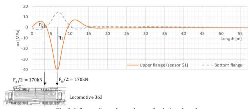
**Fig. 2.** Influence lines of normal stress for the location of sensor S1 (bridge T2-O2) and its evaluation in case of locomotive 363
