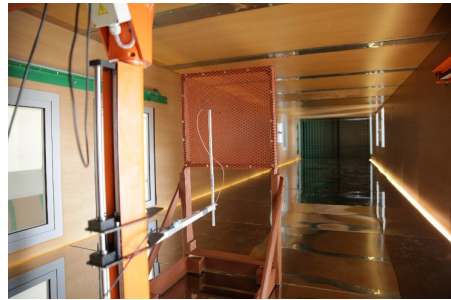
Fig. 3. HWA MiniCTA Type 54T42 mounted on traverse system
