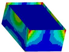
Fig. 7. Bending moments  $m_x$  as a result of seismic excitation in the direction of x-axis with the maximum value 14,561 kNm/m (red surface)
