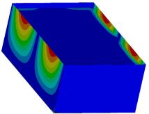
**Fig. 9.** Deformation in the direction of *x*-axis by seismic excitation in the direction of y-axis with the maximum value 0,757 mm (red surface)
