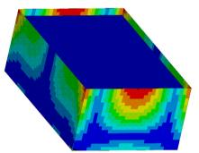
Fig. 11. Bending moments  $m_x$  as a result of seismic Fig. 12. Bending moments  $m_y$  as a result of seismic excitation in the direction of y-axis with the maximum value 8,911 kNm/m (red surface)
