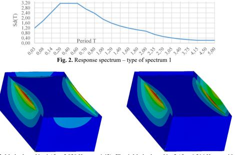
Fig. 3. Mode shape No. 1 (f = 5,920 Hz,  $\gamma = 4,42$ ) Fig. 4. Mode shape No. 2 (f = 6,216 Hz,  $\gamma = 10,68$ )
