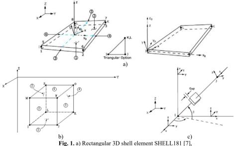
b) fluid 3D element FLUID80 [7], c) contact element CONTAC52 [7]
