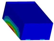
Fig. 8. Bending moments  $m_y$  as a result of seismic excitation in the direction of x-axis with the maximum value 28,021 kNm/m (red surface)
