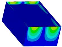
Fig. 6. Deformation in the direction of y-axis by seismic excitation in the direction of x-axis with the maximum value 0,629 mm (yellow surface)
