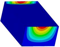
Fig. 10. Deformation in the direction of y-axis by seismic excitation in the direction of y-axis with the maximum value 2,145 mm (red surface)
