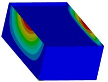
**Fig. 5.** Deformation in the direction of *x*-axis by seismic excitation in the direction of *x*-axis with the maximum value 4,785 mm (red surface)
