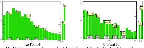
Fig. 10. 1/3-octave sound pressure level distribution on left and right sides of the corridors
