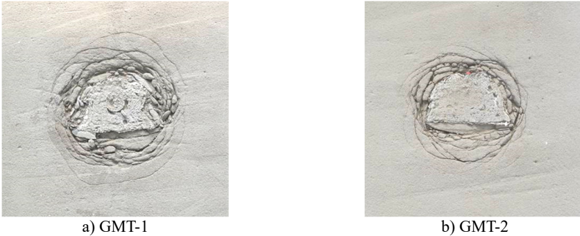
Fig. 11. Fracture distribution around excavated tunnel after axial overloading to 4.96 MPa
