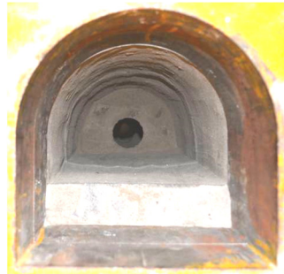
Fig. 6. Final excavated model tunnel
