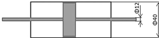
Fig. 8. Actuator used instead of classical damper
