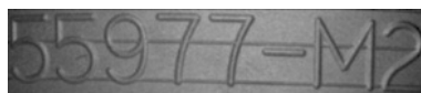
Fig. 5. Result of image segmentation for wheel hub model (55977-M2) with histogram threshold method
